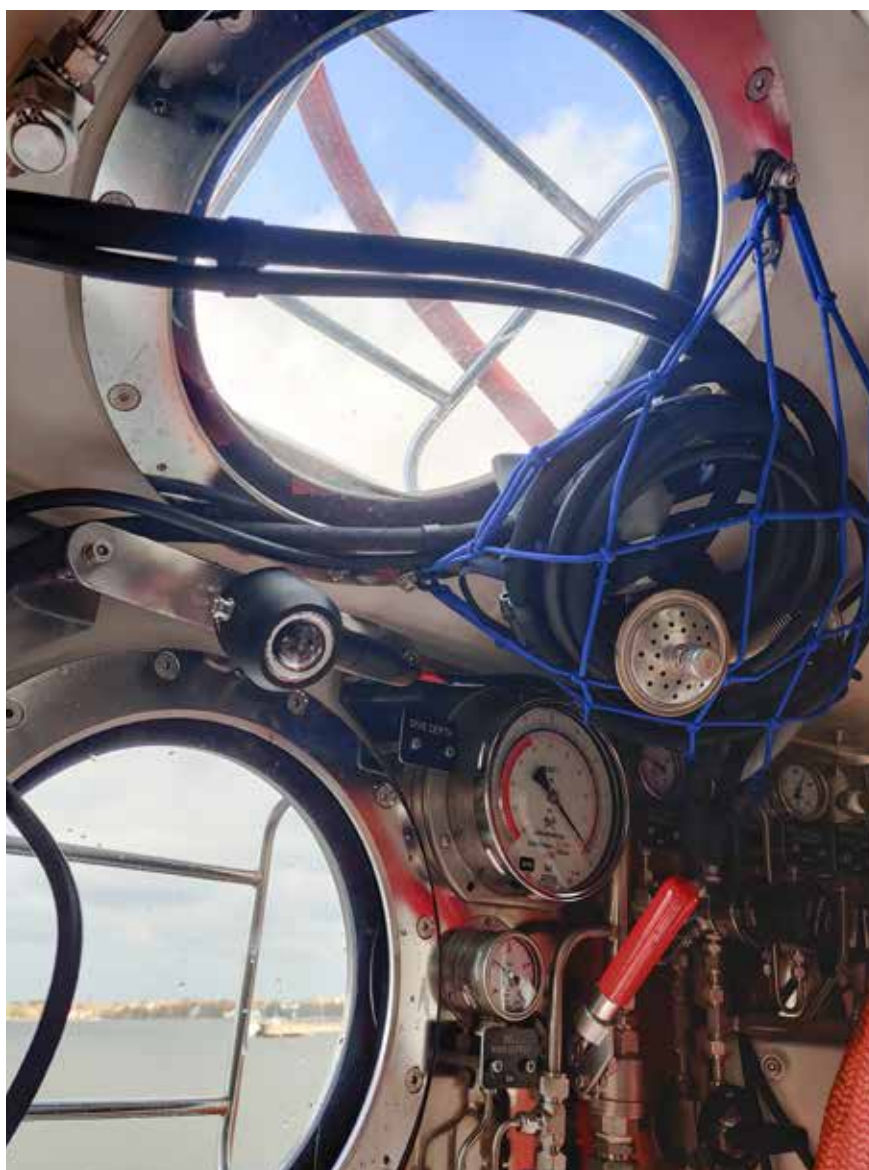
An inside view of the wet bell.
